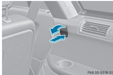
Protective cap in the right-hand side trim on the third row of seats
