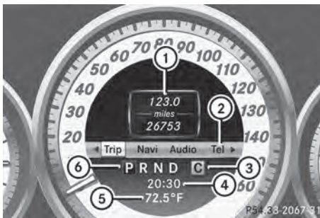
Example: multifunction display for automatic transmission
