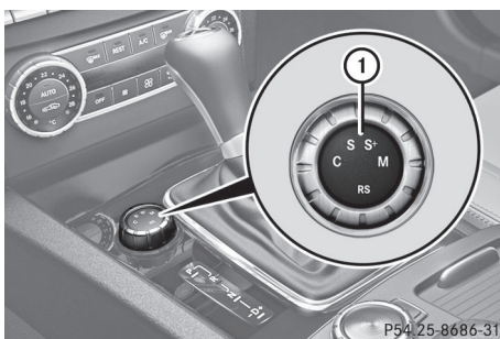
Drive program selector with manual drive program
